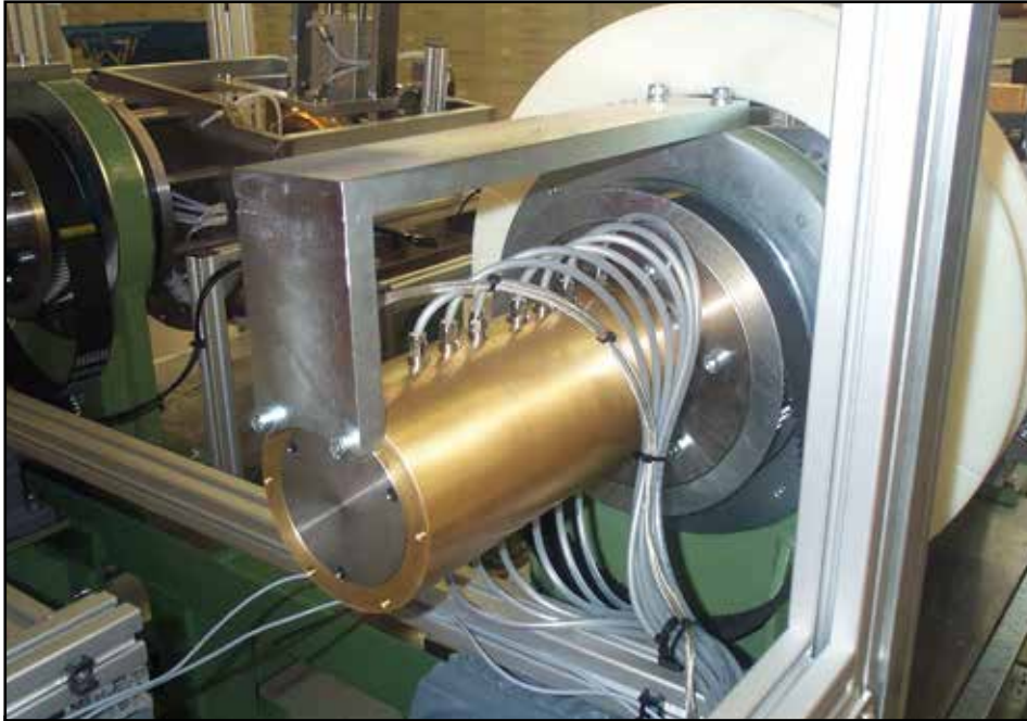
Application example: 13-passage rotary coupling with 6 connections for compressed air, 6 connections for cooling water, 1 connection for forming gas; with electronic slip ring 12 x 24V, 2A per line. For more examples refer to our catalogue or to www.hydrokomp.de .
